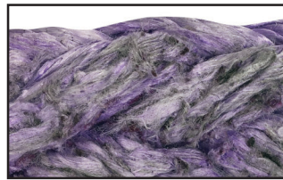
Excessive External Abrasion
